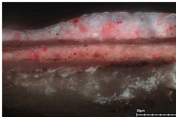
Cross-section of a microscopic paint sample from Joos Vijd's left hand. Varnish layers are clearly visible between the two pink paint layers.
