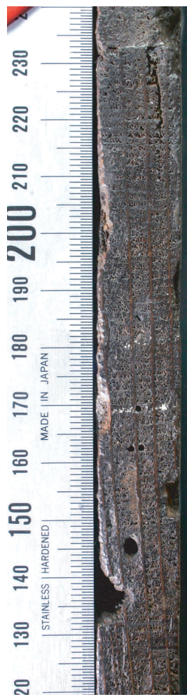
Fig. 6b. Right edge, detail (without preparation). Full quarter cutting but medullary rays slightly curved. Wood damaged.
