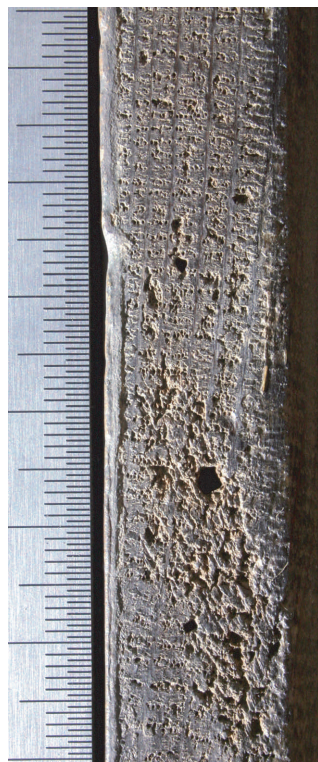
Fig. 14b. Upper edge, detail (without preparation). Full quarter cutting. Surface of plank irregular.
