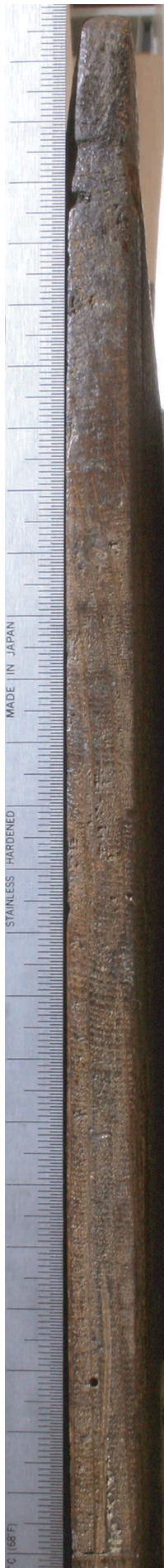
Fig. 15a. Lower edge (before preparation). Medullary rays sinuous, in particular at the start of growth (on right in the photo).
