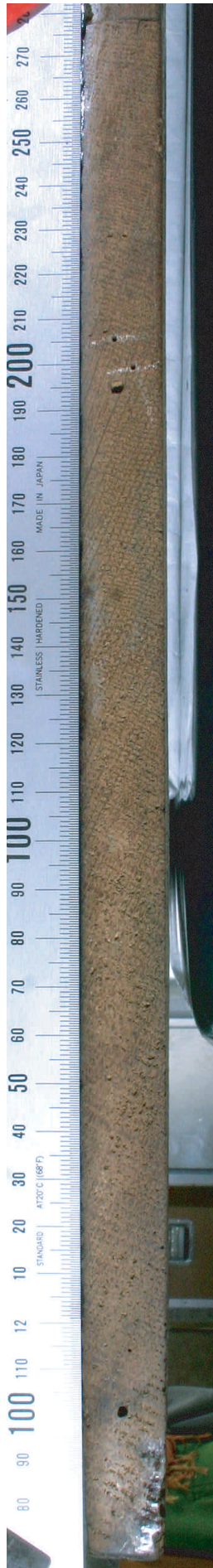
Fig. 3a. Left edge, complete view before preparation. The medullary rays are slightly sinuous, in particular at the end of growth (on right).
