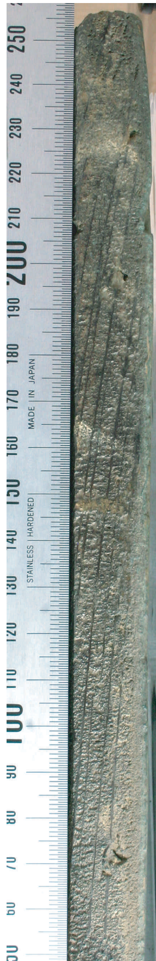
Fig. 7b. Upper edge, complete view (without preparation). Quarter cutting and medullary rays very slightly curved. Surface of the plank more irregular than on the other edge (Fig. 7a).
