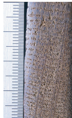
Fig. 6c. Left edge, two details after preparation (brush only). Quarter cutting. Relatively rapid growth at the start (on left) and slow at the end. Also on the right, some slight damage to the wood, which, however, does not cause problems in measurement given the thickness of the plank.
