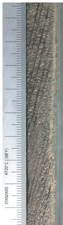
Fig. 8b. Upper edge, detail (without preparation). Quarter cutting. Surface of the plank more irregular than on the other edge (Fig. 8a).
