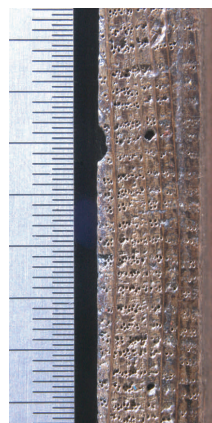
Fig. 14c. Lower edge, two details (after preparation by brushing). Full quarter cutting but medullary rays sinuous. Relatively rapid growth (in comparison with the majority of the other planks in the altarpiece).
