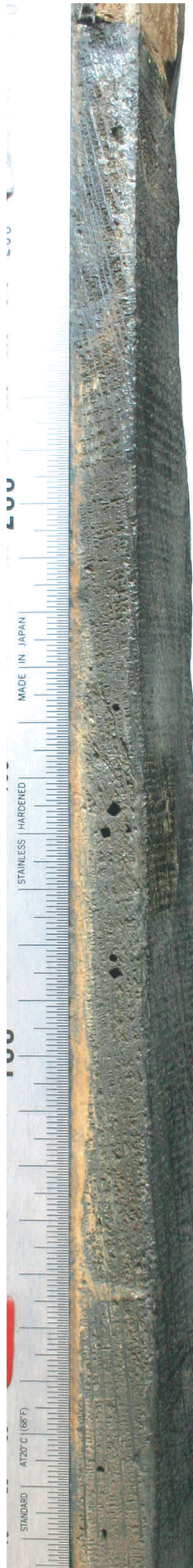
Fig. 11a. Upper edge, detail (before preparation). Medullary rays very slightly sinuous especially at the end of the sequence (left in the photo).
