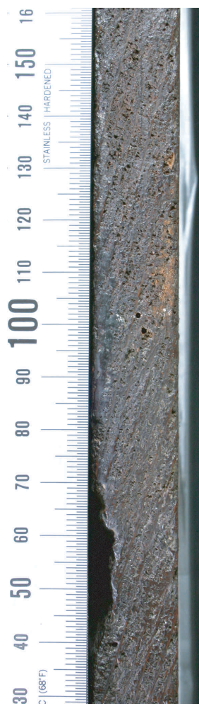
Fig. 4b. Right edge, detail (without preparation). Quarter cutting. Surface of the plank more irregular than on the other edge (Fig. 4a).
