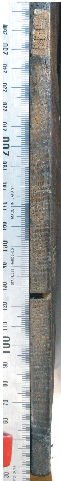
Fig. 10a. Lower edge, complete view (without preparation). Medullary rays fairly sinuous.
