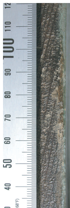
Fig. 9b. Upper edge, detail (without preparation). Quarter cutting. Surface of the plank irregular.
