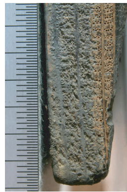
Fig. 12c. Upper edge, two details after preparation (cutter and brush). Full quarter cutting. Fairly slow and regular growth (on the right) with slowing at the end of the sequence (on the left).
