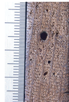
Fig. 6c. Left edge, two details after preparation (brush only). Quarter cutting. Relatively rapid growth at the start (on left) and slow at the end. Also on the right, some slight damage to the wood, which, however, does not cause problems in measurement given the thickness of the plank.
